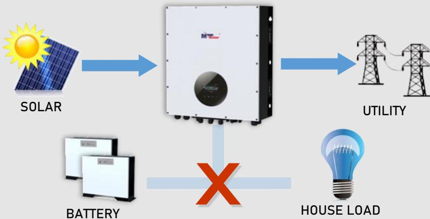
In this operation mode, the inverter will only behave like a pure grid-tie inverter where it feeds back electricity to grid from PV array.
