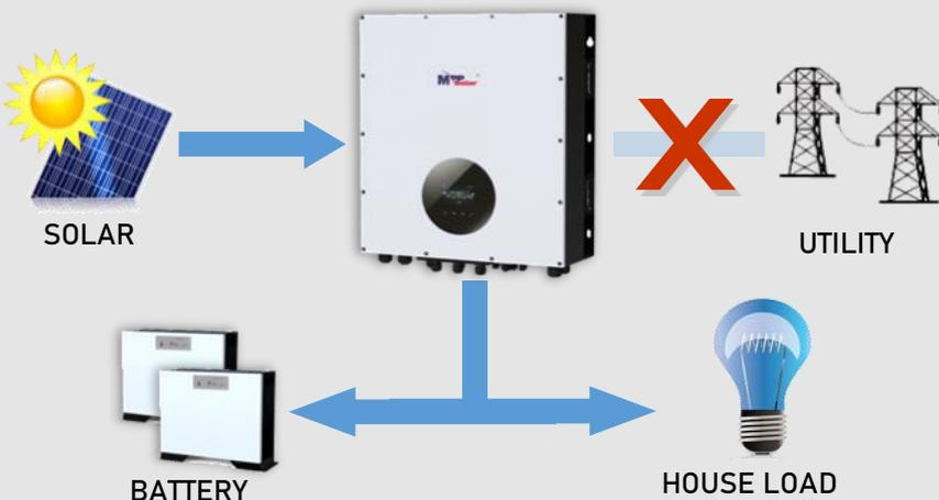
In this operation mode, grid feedback to utility is disabled. Users can only program unit to:
