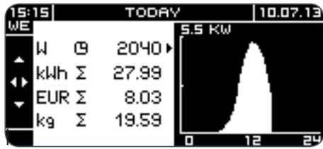
During normal operation, the operating mode is displayed. The power data is shown in a table and graph. In this way, the operation display provides an overview of the feed-in process and the yield of the PV system.
