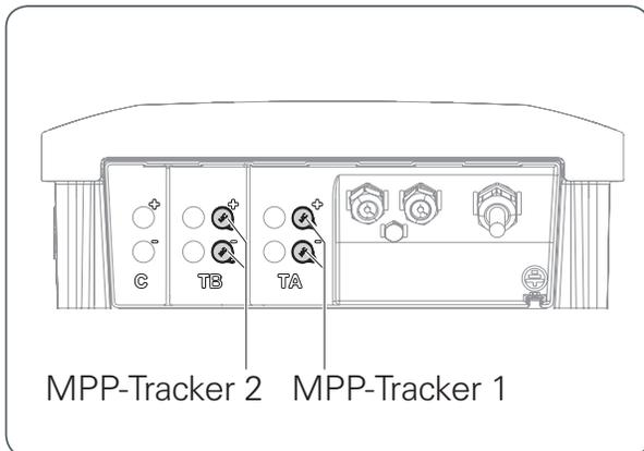
1. Furnish the DC voltage cable for every string with original Multi-Contact MC4 plugs. Make sure that the polarity is correct here.
