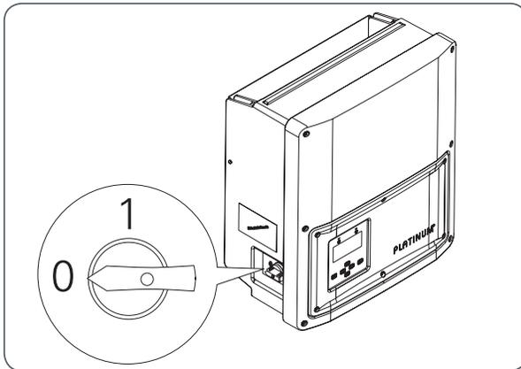
1. Move the switch knob of the DC isolator to position 0.
