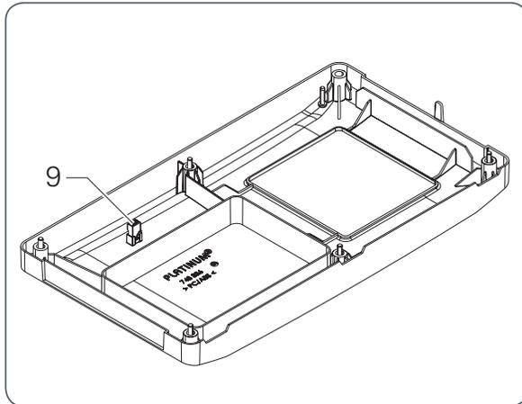
1. Remove the terminating plug (9) from the service cover.
