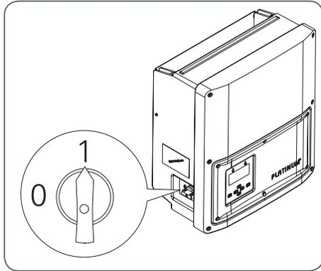
1. Switch on mains voltage supply (safety).
