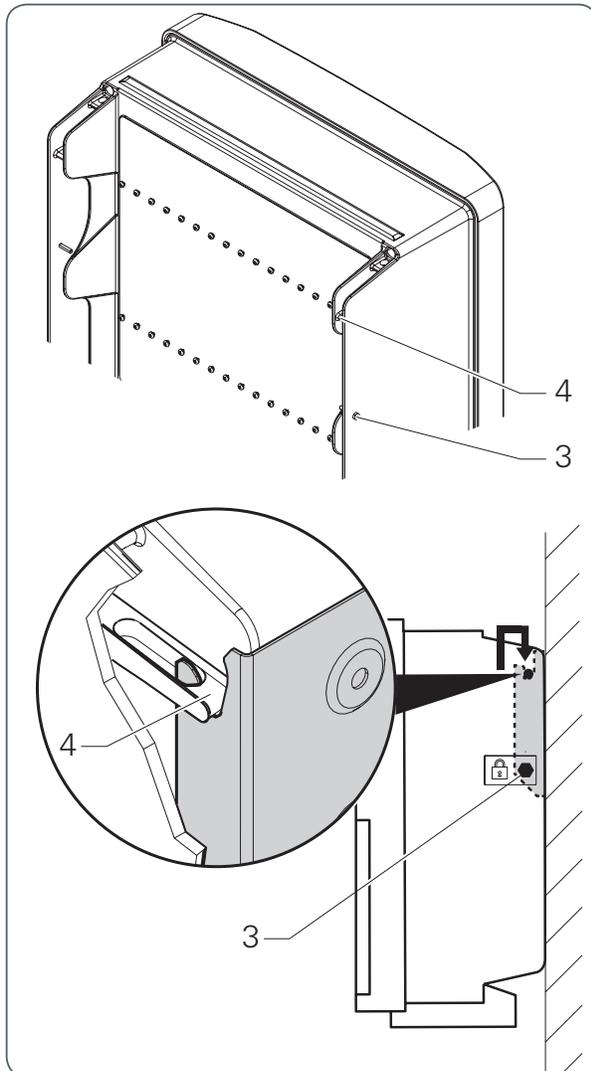
3. Loosen, but do not remove, the safety screws on the sides (3).
