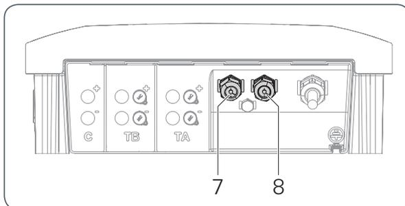
1. Unfasten the network screw connections (7) and (8) with seal from the underside of the inverter.
