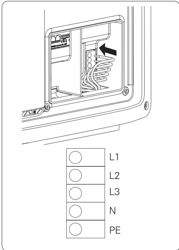
1. Unfasten the AC screw connection (6) with seal from the underside of the inverter.
