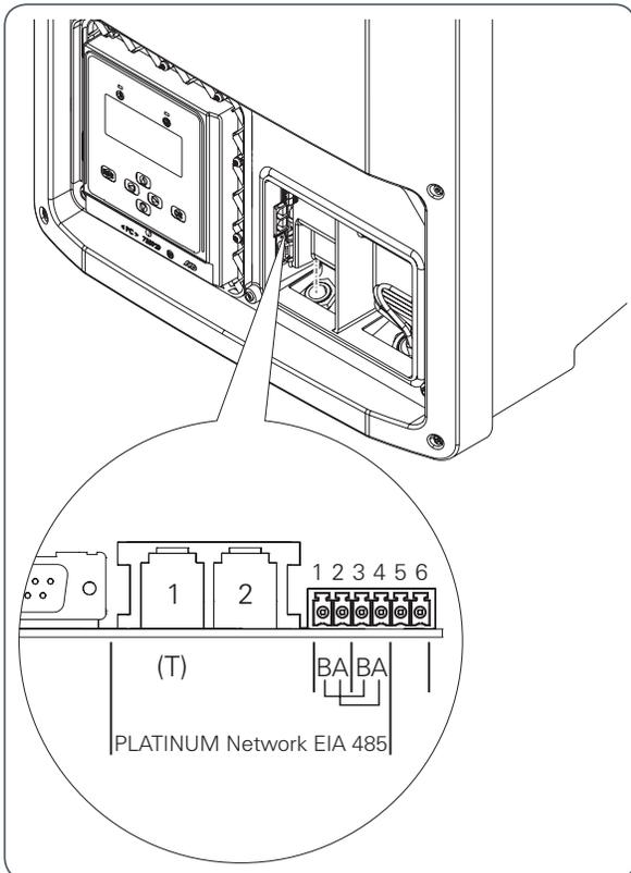
5. Connect the network cables in the inverter.
