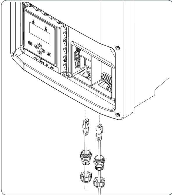
2. Direct the network cable through the screw connection and seal.
