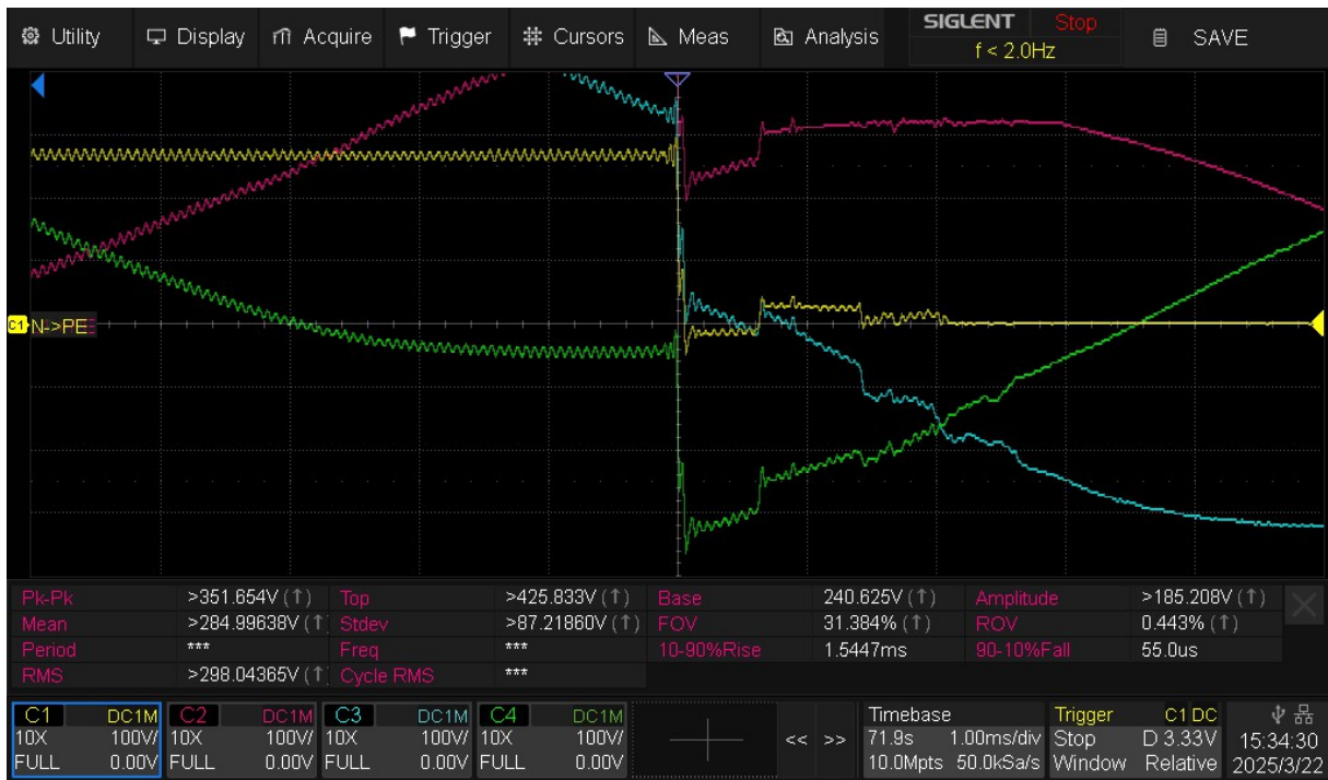
Figure 8 - Detail 4 (grid relays closing)
