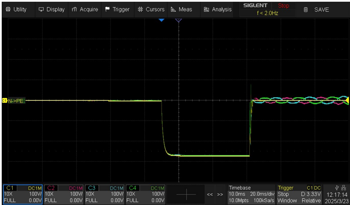
Figure 11 - Settings change (inverter restart offgrid)
