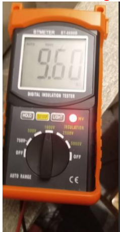
Insulation Resistance tester. In this example String 1, PV+ → 9.6GΩ
